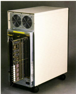
The TAAC-1 board set plugs into Sun Microsystems Workstations to speed application processing.
